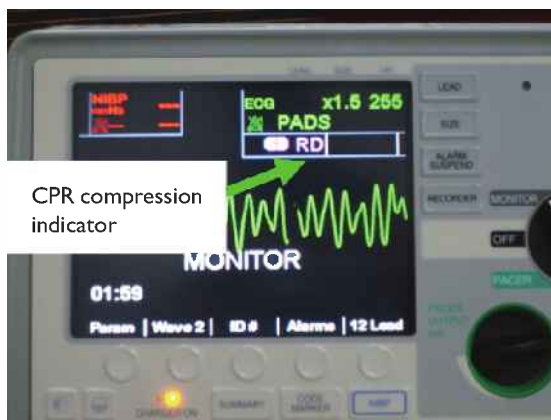
Fig. 2 Defibrillator screen display incorporating QCPR feedback indicators (Zoll E series). When complete filling of the CPR compression indicator has not been achieved due to diminished compression rate or depth, the E Series will display the letter R for rate and/or the letter D for depth to assist the rescuer in determining whether chest compression rate or depth should be increased. When appropriate rate and depth have been achieved, these letters will disappear from the display field. A voice prompt option is also available.
