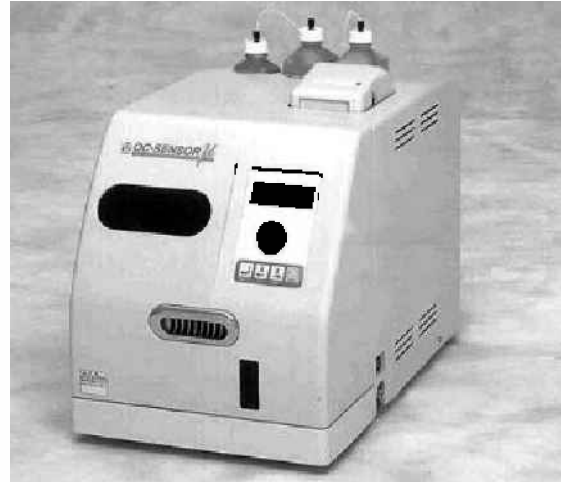
Fig. 2 Photograph shows an automated desktop machine which allows for multiple samples of faecal occult blood test kits to be analysed at the same time.
