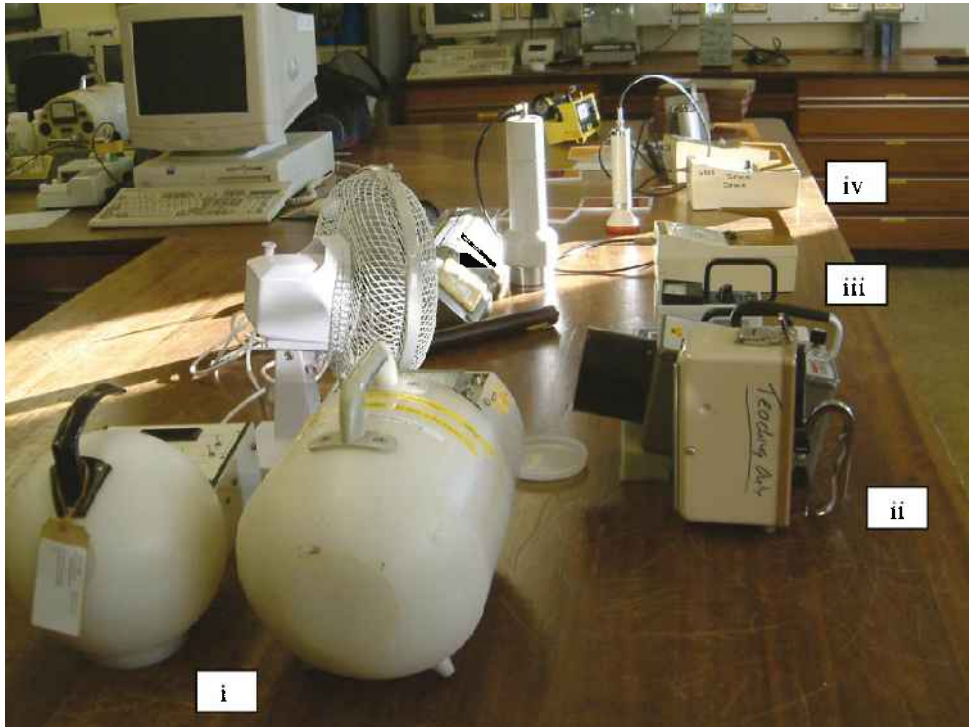
Fig. 1 Different types of dosimeters: (i) neutron detectors; (ii) gamma detector; (iii) alpha detector; and (iv) beta detector.
