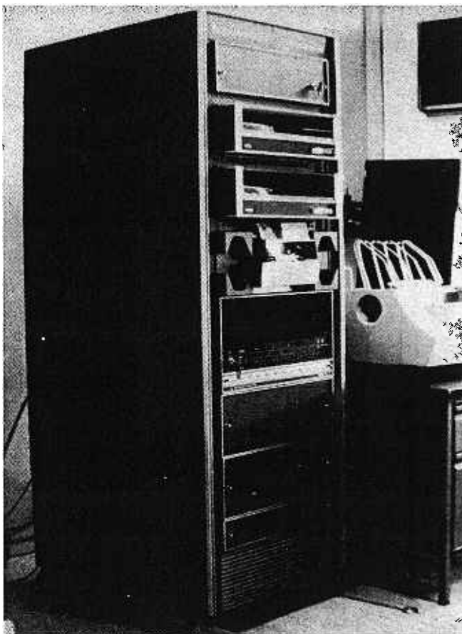
Fig. 3. Nova 1220 Central Processor with two Disc Cartridge Drives and Fast Paper-Tape Reader.
